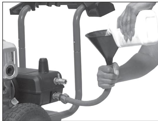
**CAUTION:** Risk of property damage. Use only RV antifreeze. Any other antifreeze is corrosive and can damage pump.
