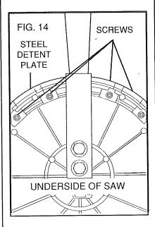
Using the carpenter's square to check your work, slide the steel detent plate as necessary to achieve squareness between the blade and fence.
