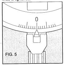
NOTE: In order to insure accuracy and repeatability, the miter pointer can be adjusted left or right as desired. To set the pointer, adjust
