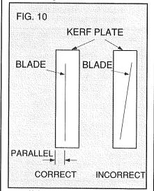
If the blade appears to be parallel, proceed to step 4, if not, loosen (do not remove) the two pivot mount bolts under the back edge of the saw table that hold the pivot mount (see Fig. 11) to the saw. Align the blade as necessary and tighten the pivot mount bolts (280-320 in. lbs.). (DO NOT OVERTIGHTEN.)
