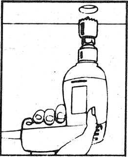
HOLE SAWS will cut larger diameter holes in wood up to 3/4" thick.
