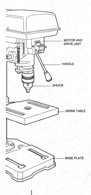
Tilt the table as desired and align the "0" mark on the table with the appropriate mark on the scale. Tighten the bolt to hold the table at the desired angle.
