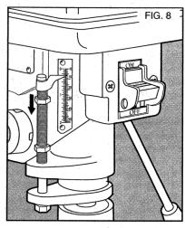
Lock the nut in place by screwing the top hex nut down against the lower one. Release the handle letting the chuck rise to its full height.
