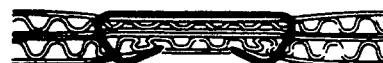
Staple driven completely through two thicknesses of corrugated board and clinched on underside.
