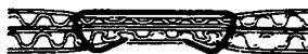
Staple driven completely through two thicknesses of corrugated board and clinched on underside.
