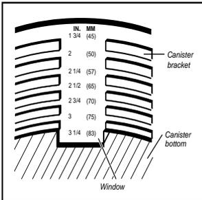
3. **Load the coil of nails:** Place a coil of nails over the post in the canister. Uncoil enough nails to reach the feed pawl, and place the second nail between the teeth on the feed pawl. The nail heads fit in slot on nose.
