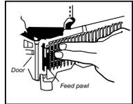
1. **Open the magazine:** pull down down latch and swing door open. Swing magazine cover open.
