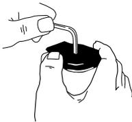
Loosen screw as shown. Adjust to desired exhaust direction and tighten screw.
