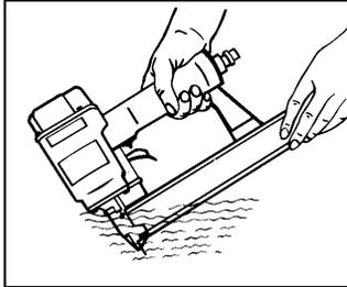
Tar and dirt may build up on the nose and contact arm. This can prevent correct operation. Remove any buildup with kerosene, #2 fuel oil or diesel fuel. Do not immerse the stapler into these solvents beyond the bottom of the frame to avoid getting the solvent into the drive cylinder.
