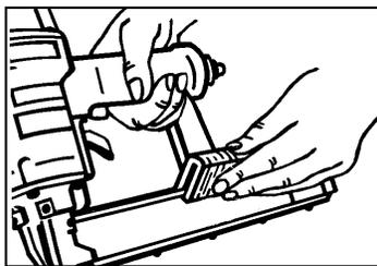
2. Use stick of staples to move cover spring to one side and drop over core of magazine. Repeat until magazine is loaded, allowing enough space for pusher to disengage from the latch.
