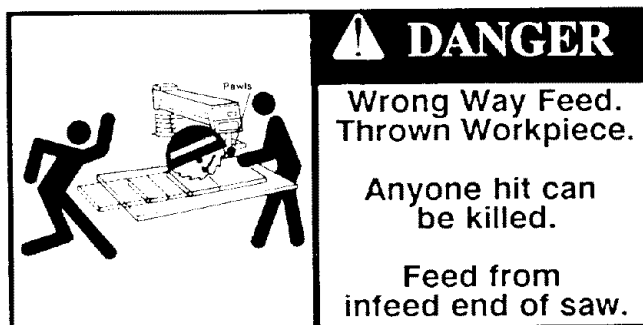
Fig. 100 Wrong Way Feed Safety Signs
