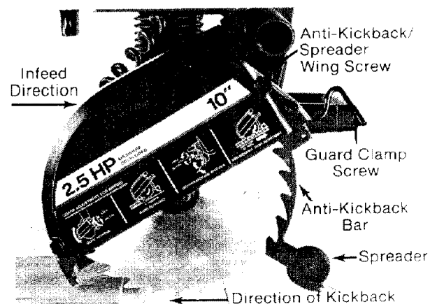
Fig. 103 Blade Guard Position for Ripping
