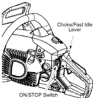
1. Move ON/STOP switch to the ON position.
