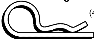
(4) Retainer Springs (double loop)
