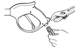
6. Connect high pressure hose to outlet on pressure washer and hand tighten firmly.
