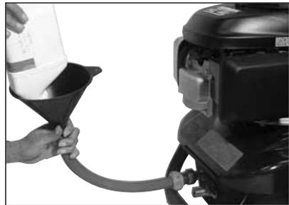
6. Pull engine starter rope slowly several times until antifreeze or windshield washer fluid comes out of high pressure hose connection of pump.
