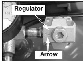
7. Reapply pipe sealant to gauges and quick connect.
