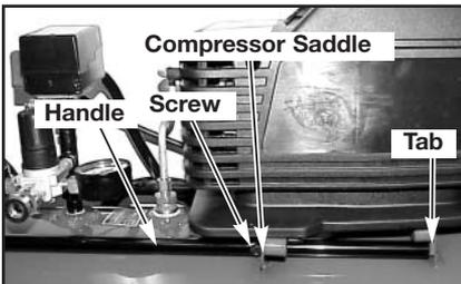
**CAUTION** It will be necessary to brace or support one side of the outfit when installing the wheels because the compressor will have a tendency to tip over.
