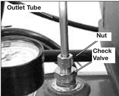
4. Unscrew the check valve (turn counterclockwise) using a socket wrench.
