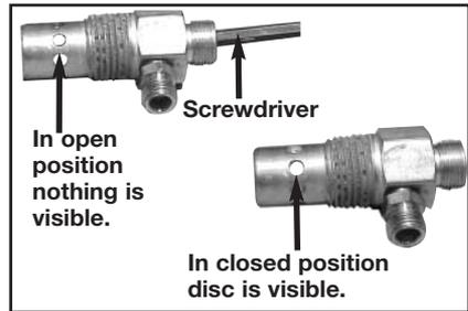
6. Apply sealant to the check valve threads. Reinstall the check valve (turn clockwise).
