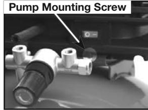
8. Apply pipe sealant to new regulator manifold and assemble, tighten with wrench.
