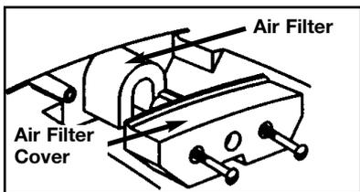
2. Remove the air filter and make sure it is clean.
