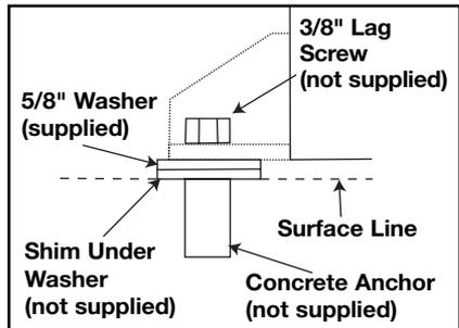
3. Line-up holes in surface with holes in air compressor feet.
