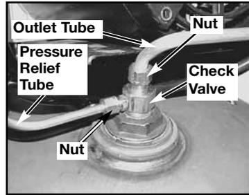
7. Unscrew the check valve (turn counterclockwise) using a 7/8" open end wrench. **Note** the orientation for reassembly.
