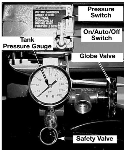
**On/Auto/Off Switch:** Turn this switch ON to provide automatic power to the pressure switch and OFF to remove power at the end of each use.
