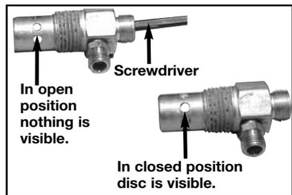
9. Clean or replace the check valve. A solvent, such as paint or varnish remover can be used to clean the check valve.
