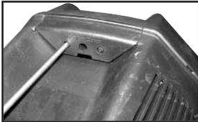
4. Remove the rear shrouds using T-20 torx wrench.
