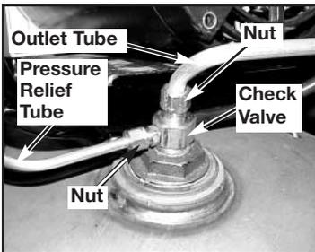
5. Using an adjustable wrench loosen pressure relief tube nut at air tank and pressure switch. Carefully move pressure relief tube away from check valve.
