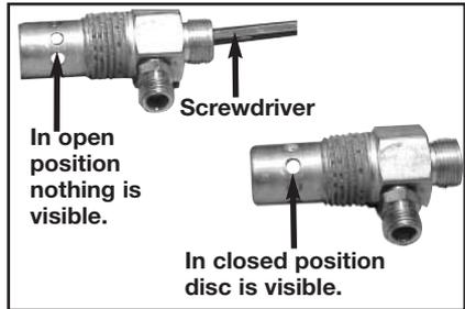
8. Clean or replace the check valve. A solvent, such as paint or varnish remover can be used to clean the check valve.
