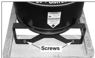
**CAUTION** It may be necessary to brace or support one side of the air compressor when removing the pallet because the air compressor will have a tendency to tip.
