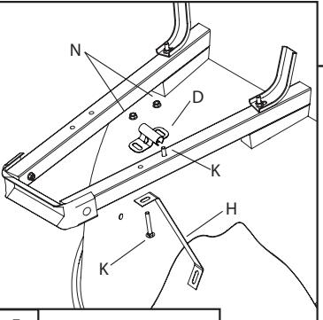
**6** Attach axle bracket (D) to bottom of handle using a bolt (K) pushed through the hole closest to tray. Push second bolt (K) through hole in bottom of tray brace (H) then through handle (using hole closest to wheelguard) and finally through axle bracket. Attach loosely with nuts (N). Repeat to attach second axle bracket to other handle.
