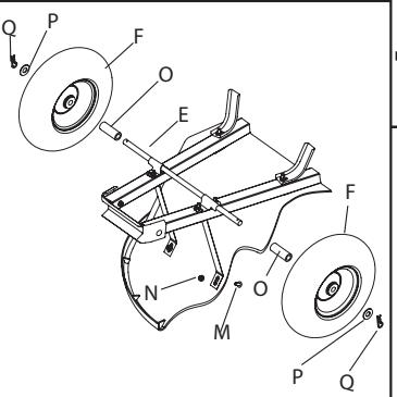
**7** Slide axle (E) through both axle brackets. Slide spacer (O), wheel assembly (F) and washer (P) onto end of axle. Secure by attaching cotter pin (Q) through hole in end of axle. Repeat to attach second wheel. Use bolts (M) and nuts (N) to attach tops of tray braces to tray.
