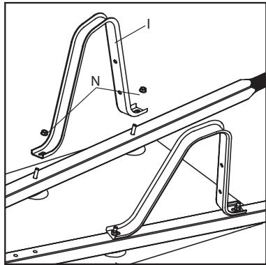
**3** Make sure the holes in leg (I) are facing the back of the tray and then place leg over bolts and loosely attach to handle with nuts (N). Repeat for other leg.
