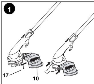
**⚠ WARNING:** To avoid serious injury, never use the tool unless the guard is properly fitted.
