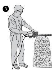
3 TRIMMING NEW GROWTH - (Figure 4) – A wide, sweeping motion, feeding the blade teeth through the twigs is most effective. A slight downward tilt of the blade, in the direction of motion gives the best cutting.
