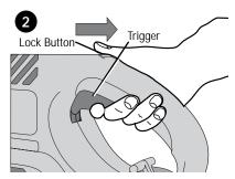
TO LOCK THE TOOL ON FOR CONTINUOUS RUN WITH THE TOOL RUNNING, pull the LOCK BUTTON ALL THE WAY back, release the TRIGGER, then release the LOCK BUTTON. The tool is now locked ON. To turn the tool OFF, squeeze and release the TRIGGER. NOTE: In order to lock the tool on, it is important to first release the trigger and then release the lock button.
