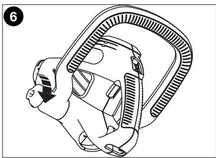
**NOTE:** The handle on the 79442, 51891 is adjustable to three different positions as shown **figure 7**. To move handle, unscrew plastic knob, position handle as desired and retighten knob.
