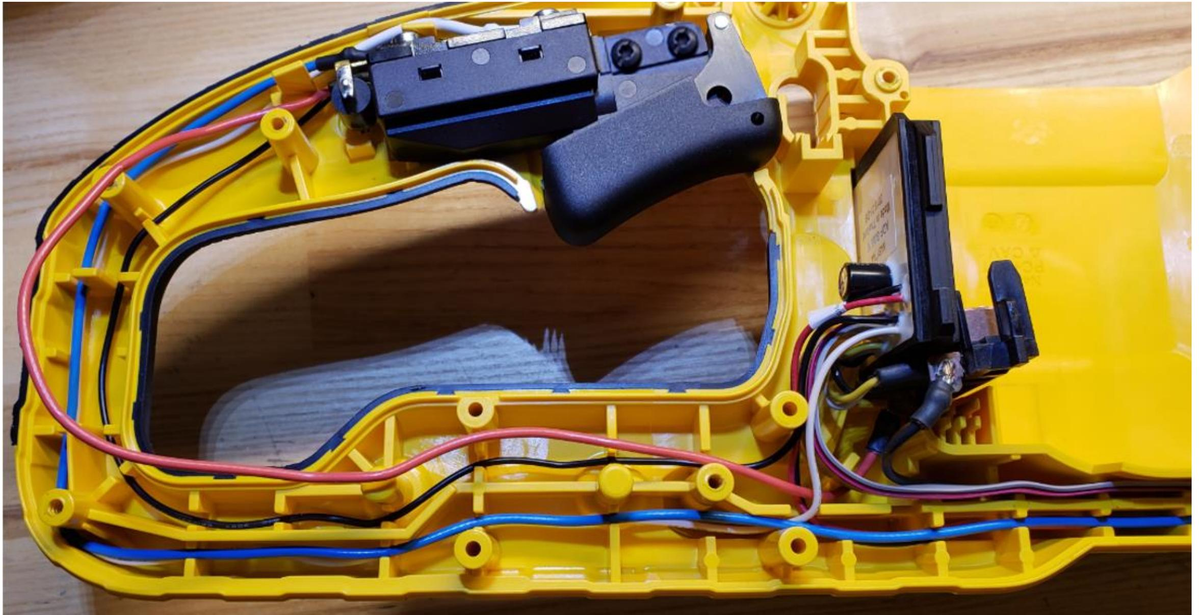
Finish routing Black Power Wire into Assembly Housing wire ways, retaining Red Signal Wire as you go.
