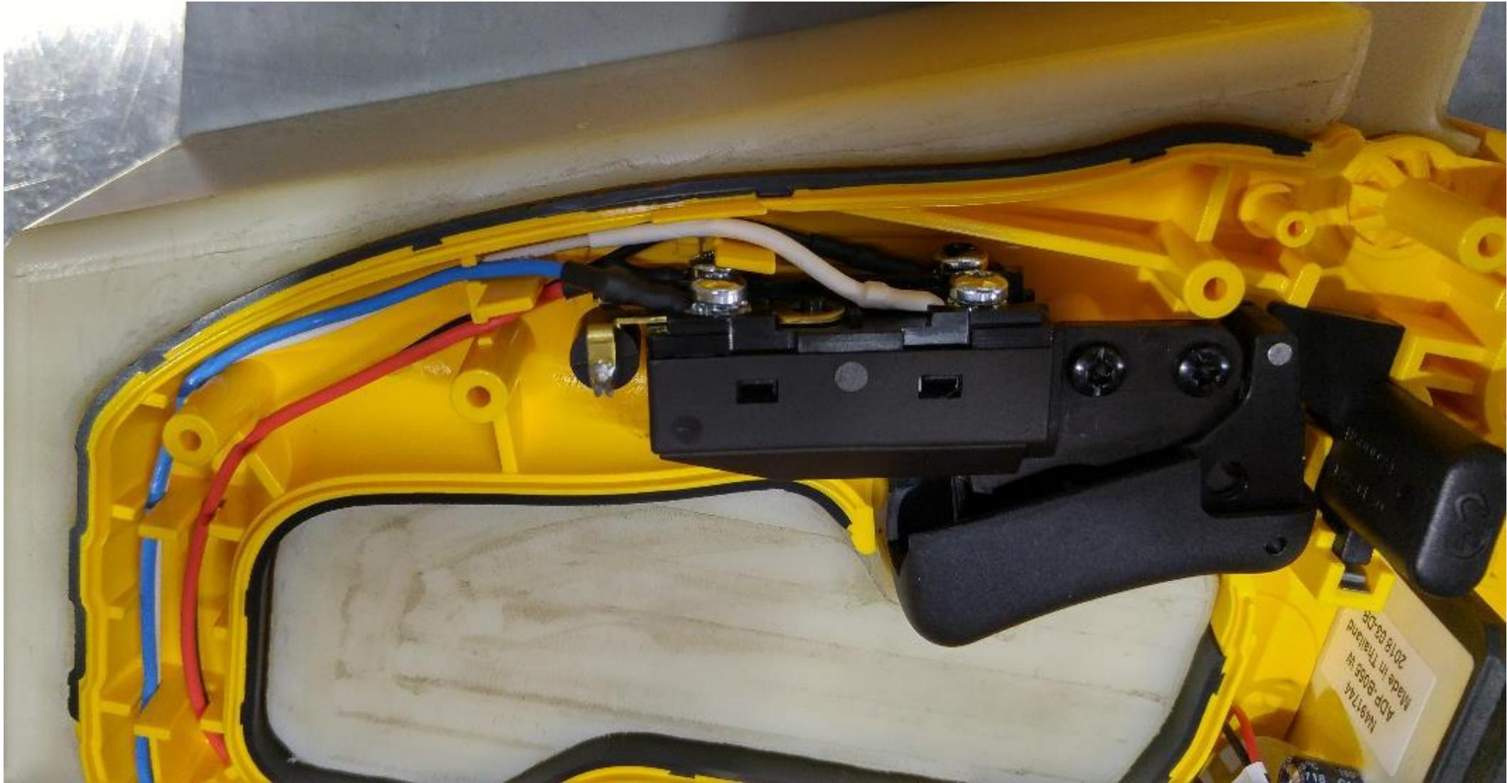
Finish routing Blue Power Wire into Assembly Housing wire ways, retaining White Signal Wire as you go.
