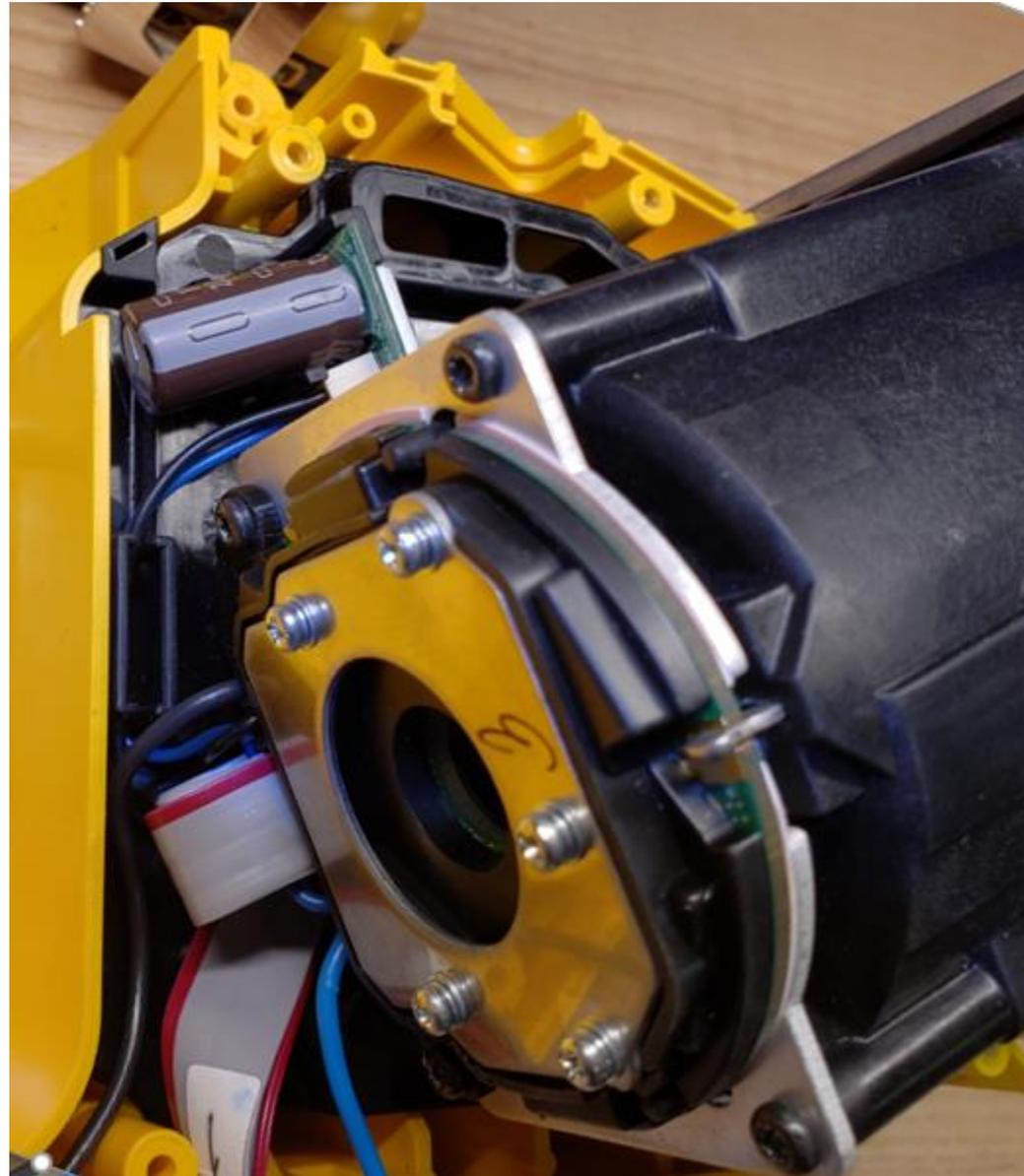
Route Capacitor wires into Intermediate Plate wire traps as shown,
