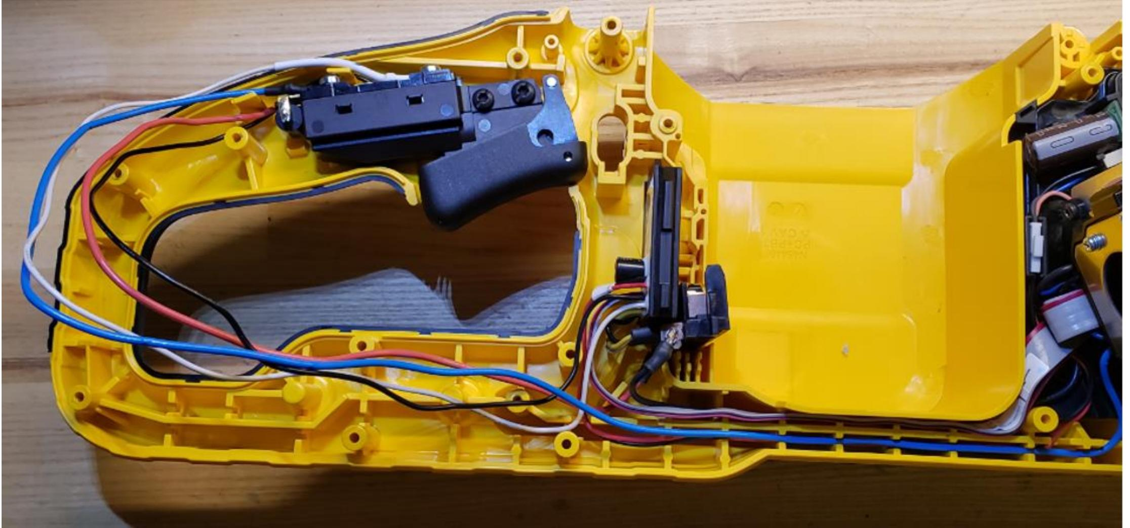
Route White Signal Wire in Assembly Housing wire ways as shown.
