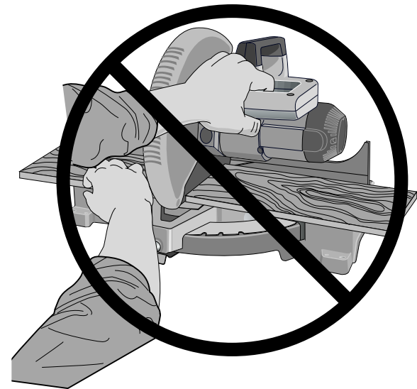
IMPROPER HAND POSITION
