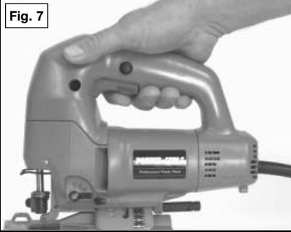
Choose a convenient starting point. Hold the bayonet saw over the point and inside the line of waste. Tip the machine forward until the front edge of the base rests firmly on the surface of the workpiece with the tip of the blade clear of the work surface, (Fig. 8).
