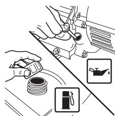
**CAUTION** Keep fuel out of the reach of children. Never fill fuel tank completely. Fill tank to 1/2" below the bottom of the filler neck to provide space for fuel expansion. Wipe any fuel spillage from engine and equipment, and make sure area is dry before starting engine.
