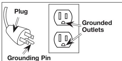
**⚠DANGER:** Risk of Electrical Shock. IMPROPER GROUNDING CAN RESULT IN ELECTRICAL SHOCK.
