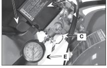
its "cut-out" pressure setting, the safety valve will protect against high pressure by "popping out" at its factory set pressure (slightly higher than the pressure switch "cut-out" setting).
