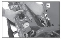
Connect air hose (sold separately) to quick connect plug (b) and quick connect
