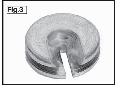
To install insert, remove saw blade from Bayonet Saw and locate insert in the throat of the saw base with the slot forward and the beveled side of the slot up. Install appropriate blade as outlined in section INSTALLING THE BLADE with the blade body in the slot of the insert. To unlock the lock button, squeeze trigger allowing lock button free to spring out, and release.
