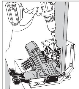
Ensure drill collar plate is fully pushed down by drill.
