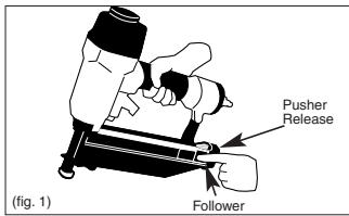
Insert nails into track of magazine
